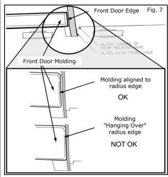
9) Align rear edge of Front Body Side Molding to radius on rear edge of front door as shown in Fig. 7.
