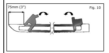
13) Peel back tape liner 75 mm (3") from all 4 ends, as shown in Fig. 10.
