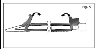
7) Remove tape liner from both ends of Front Body Side Molding, as shown in Fig. 5.
