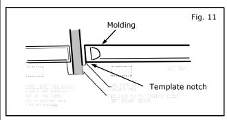
14) Align front edge of Rear Body Side Molding to template notch as shown in Fig. 11.
