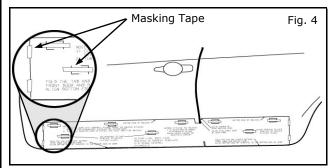
6) Secure template with masking tape. (See Fig. 4)
