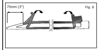
8) Peel back tape liner 75 mm (3") from both ends, as shown in Fig. 6.
