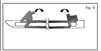
12) Remove tape liner from both ends of Rear Body Side Molding, as shown in Fig. 9.
