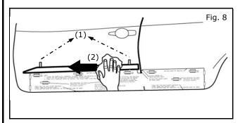
10) Align bottom edge of Front Door Molding to top edge of template and press lightly into postion. Slowly remove tape liner from Body Side Molding. (See Fig. 8, Step 1)
